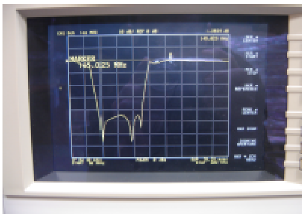
Insertion loss@145 MHz (-0.35dB)
