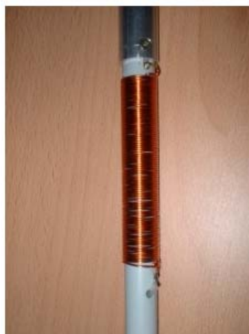
14 MHz coil (1mm CuL for 100W Tx power)
