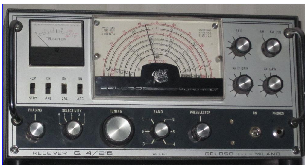
Geloso G.4/216 receiver (AM/CW/SSB)
